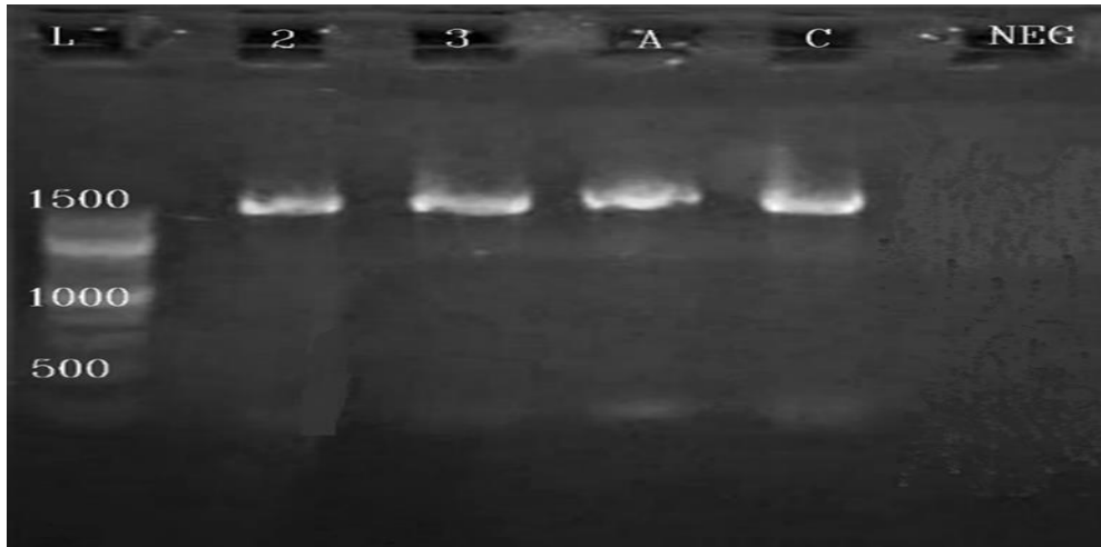
Plate II: Electrophoresis gel of 16s rRNA gene banding pattern of selected bacteria isolates Key: L: ladder, 2, 3, A, C: electrogenic bacterial isolates, Neg: negative control
